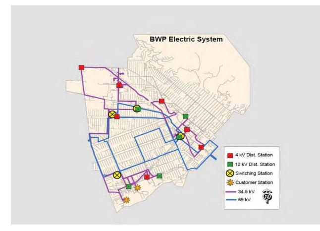
**Figure 3.15 – BWP's Electric Distribution System** Source: BWP
