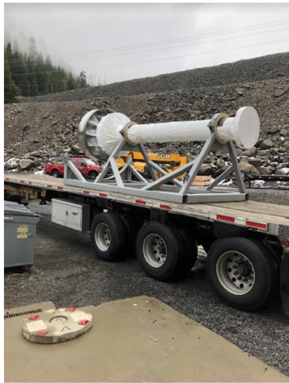
Unit 2 Turbine Shaft Transport
