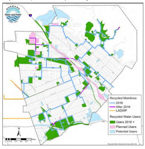
Figure 5-1: Existing Recycled Water System
