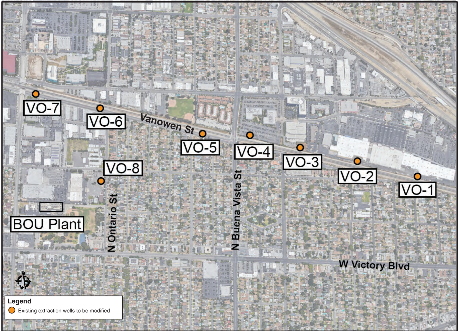
Figure 6 Existing Extraction Wells to be Modified
